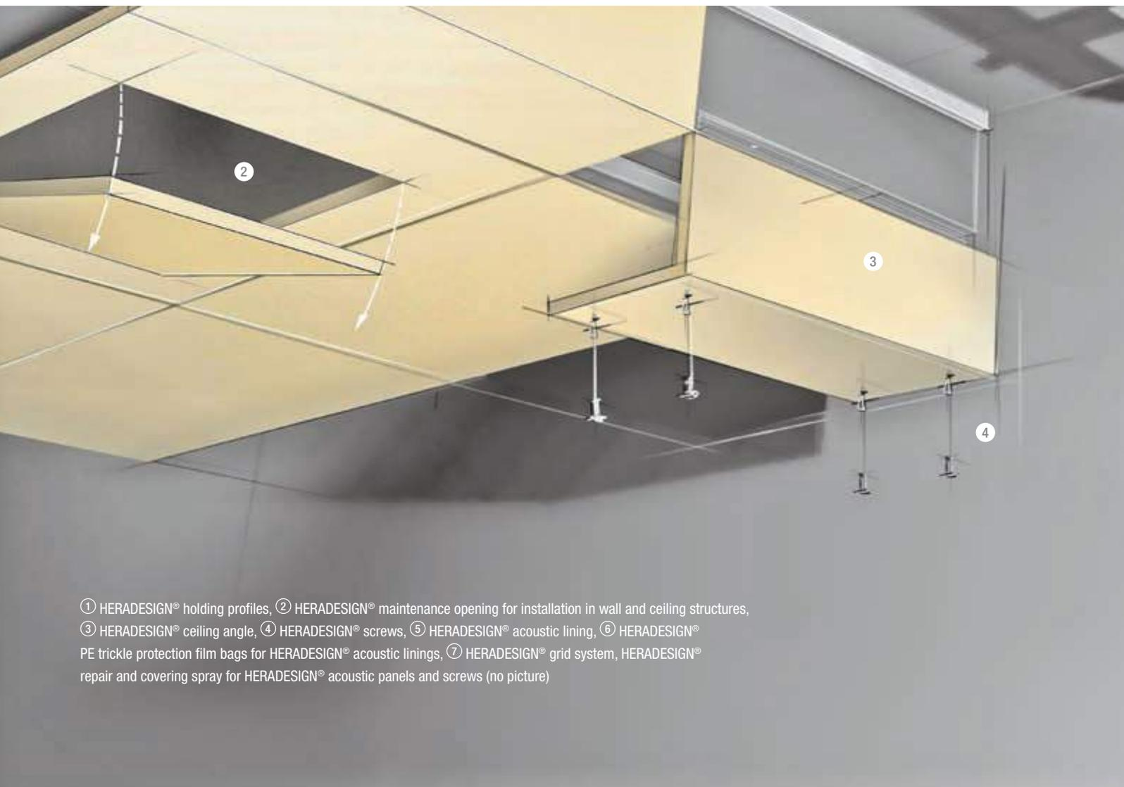
① HERADESIGN® holding profiles, ② HERADESIGN® maintenance opening for installation in wall and ceiling structures, ③ HERADESIGN® ceiling angle, ④ HERADESIGN® screws, ⑤ HERADESIGN® acoustic lining, ⑥ HERADESIGN® PE trickle protection film bags for HERADESIGN® acoustic linings, ⑦ HERADESIGN® grid system, HERADESIGN® repair and covering spray for HERADESIGN® acoustic panels and screws (no picture)
